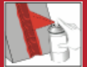
Apply penetrant on a clean, dry surface. let stand for >5 min
