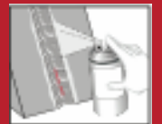
Shake the developer and apply 2 or 3 light applications
