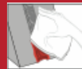
Wipe off surface penetrant
